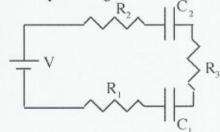
9) [8 PTS] Solve for the unknown source voltage and the power delivered by the unknown battery in the diagram below. The current through R<sub>1</sub> is 1 Ampere while R<sub>1</sub> = 9  $\Omega$ ,  $R_2$  = 3  $\Omega$  and  $R_3$  = 1  $\Omega$ . Note: A correct setup is worth 6 pts.
