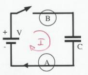
current will flow around entire circuit. Entrent is not restricted to flow on just the top or bottom
